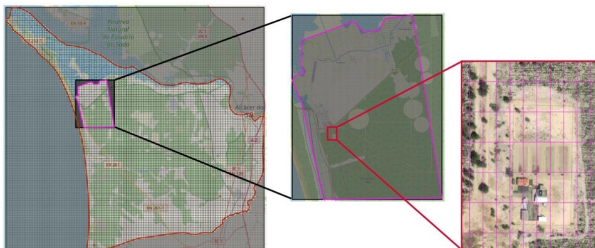
Figure 12 Regional groundwater flow model (left) and local groundwater flow model (center and right for the detail of the WWTP) for Comporta field site area.
